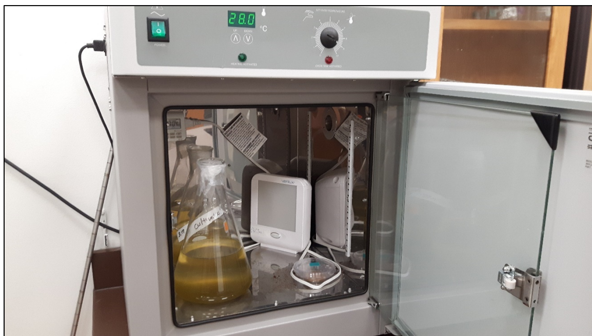
Figure 3.3. Verilux VT 10 Lamp - 5000 lux 34 (Verilux, VY), white UV light, shown in the incubator together with a Petri dish and two cell Mass Cultures.
