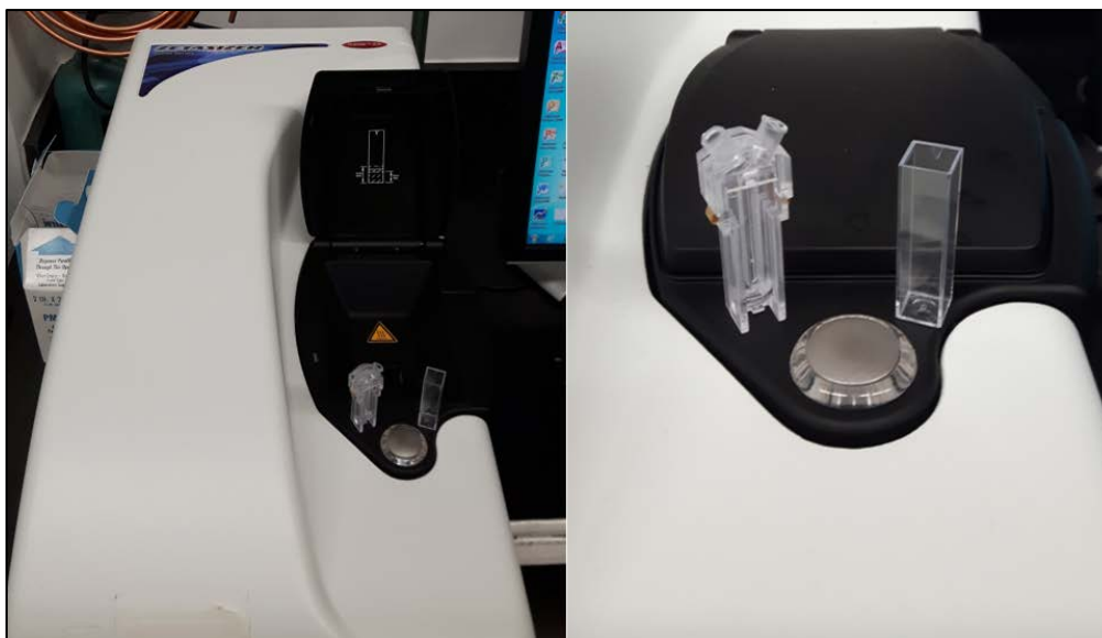
Figure 3.2. Nano ZS90 zeta-sizer 33 (Malvern Instruments, UK), and the special cuvettes used to measure zeta potential (left) and particle size (right).
